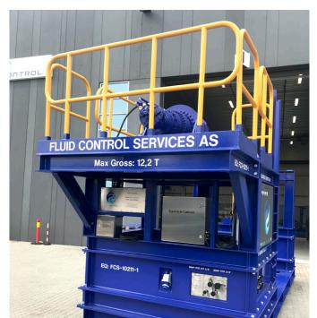
The spooler has been modified to accommodate a split drum with live centre shaft and swivel suitable for deployment/recovery of both 4" Soluforce and 2" Black Eagle hoses.
