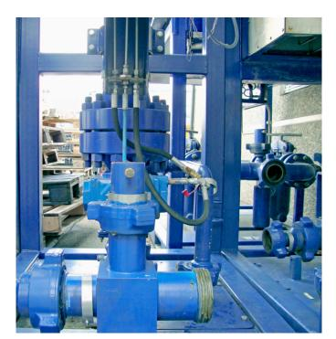
Plunger pumps and pulsation dampeners go hand in hand.
