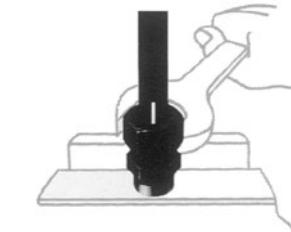
Tighten nut 1 1/2 turns if using the fitting body (1 1/4 turns if using the hardened pre-assembly tool). The tube must not turn with the nut. The stop edge in the progressive ring limits over tightening by sharply increasing the tightening torque.
