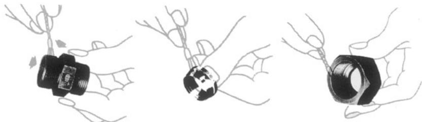
Lubricate thread and cone of fitting body or hardened
