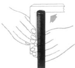
The tube is cut at a right angle.
